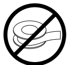
Pipe tape is not recommended.
