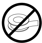
Pipe tape is not recommended.
