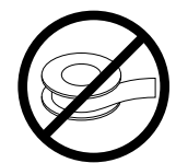
Pipe tape is not recommended.
